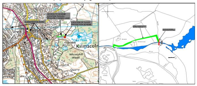
**Proposed Operations:** Construction of an earth bund with v-notch weir to control flows and increase attenuation.
